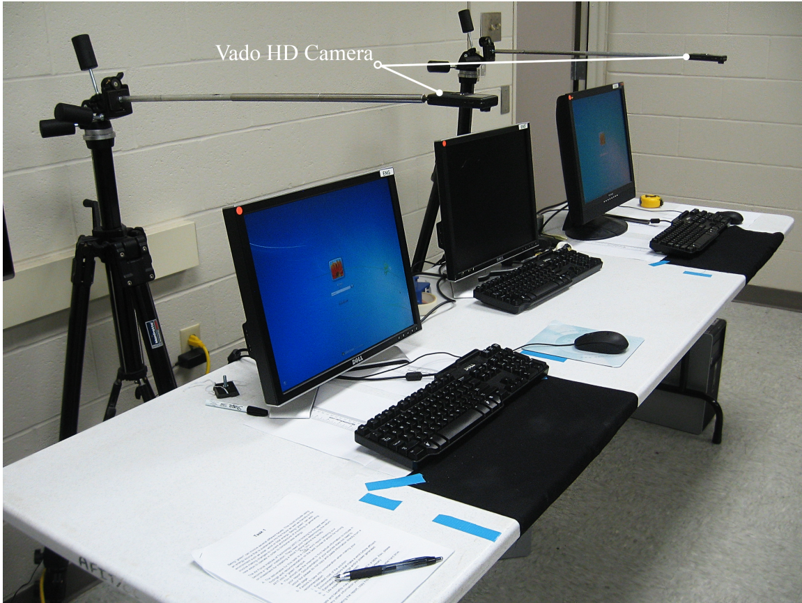
Figure 5. Photograph of the laboratory setup for two users. Both workstations have an identical setup, aside from the monitors. The Vado HD camera is connected to a tripod 54 cm above the table via a metal rod, allowing the camera to record typing without disrupting the user. A black cloth is placed underneath the keyboard for better contrast between hand and background during background subtraction. Blue tape on the table delineates for the user the approximate frame of view of the Vado camera to help the user keep other objects outside of this field of view.
